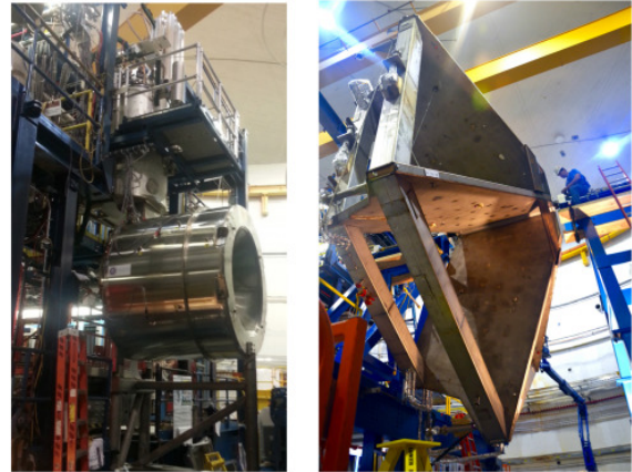
Figure 4: CLAS12 Magnets. Left: Solenoid. Right: Torus Magnet
